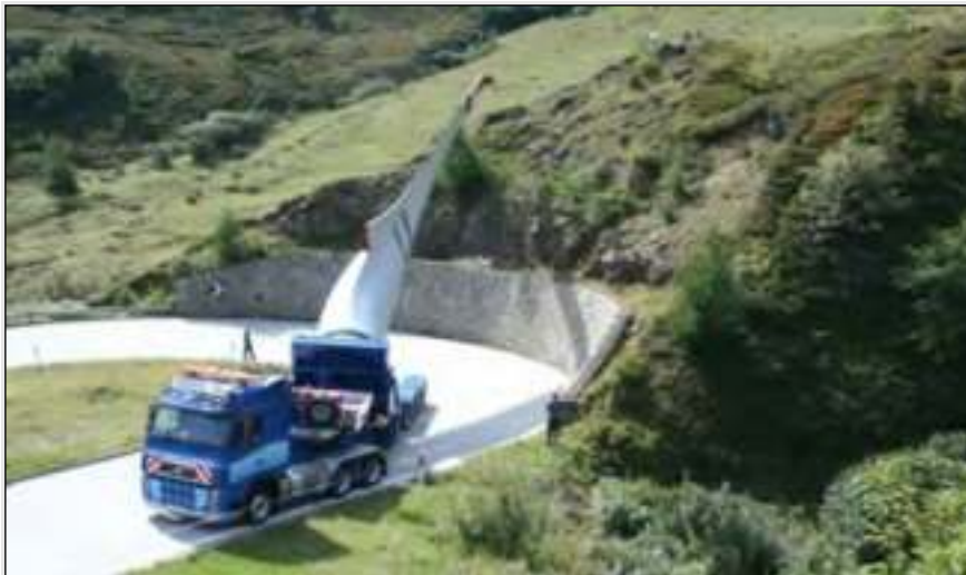
Plate 4-4 Blade adaptor transport system
